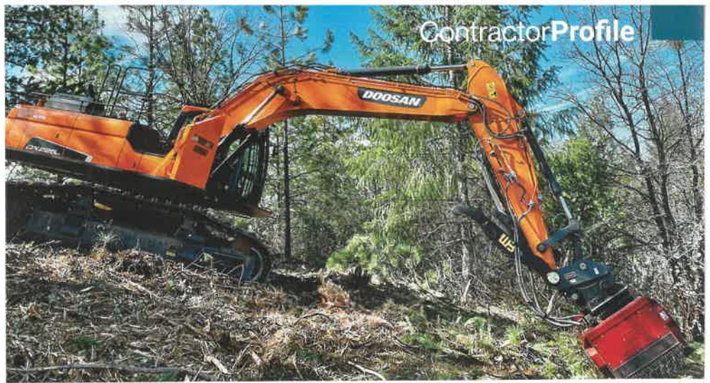
Doosan 225 Road Builder at work with a Fecon BH-40 masticator attachment. High Sierra Timber Management can provide a wide range of services, such as traditional timber harvesting, thinning, clearing utility corridors, and wildfire mitigation.
